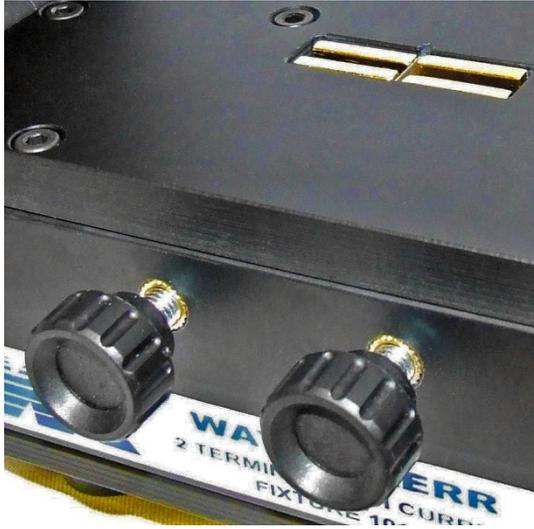
*Device Under Test mounting location*
