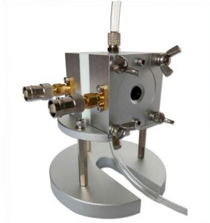
The 1J1022 Liquid Fixture is used to make accurate dielectric constant and impedance measurements of liquid materials. When used with a Wayne Kerr 6500 analyzer then the 1J1002 4-2 BNC Converter (available separately) must also be used.
